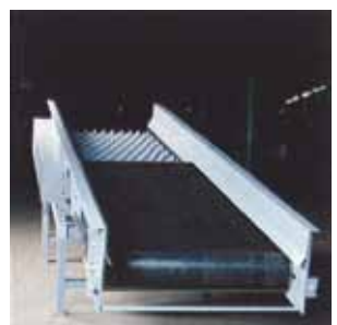
Disc screen combined with a conveyor belt.
