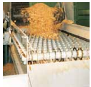
Disc screen in a chipper canter line.
